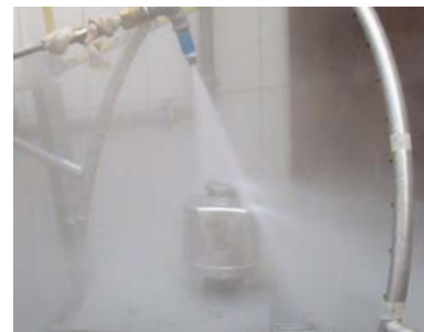
POWERCELL PDX load cells have surpassed rigorous testing for high-pressure spraying and water submersion.
