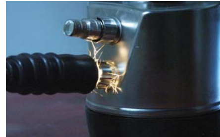
POWERCELL PDX load cell under laboratory testing of a simulated lightning strike.
